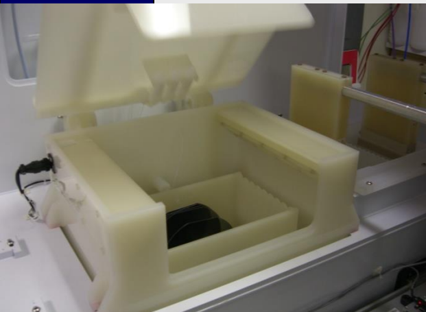
Wafers in DryZone, auto lid closing
